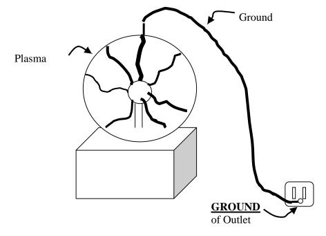
Figure 1: Ground wire used to hold a vertical streamer in place for examination of its spectrum
